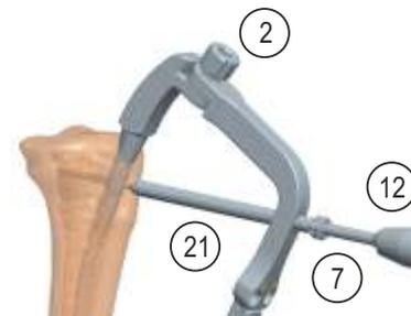
The side locking can be done through the aiming arm attachment (3). Whether we use it for the right or left tibia we insert the attachment (5) according to the „L” or „R” sign to the aiming arm (5) and we can fix them by clamp screw (6).
